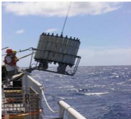
Scientists on the R/V Kilo Moana oceanographic research ship lower a rosette holding 24 bottles that capture samples at different ocean depths in the Pacific Ocean.
